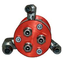
The Series 130 Valve Block Tool is the interface between a manual or automatic clamping mechanism and the fill system. Standard design includes a 3/8" NPT female connection for any manual coupler, power coupler or an automatic clamping mechanism. Refer to product bulletins, PB114 for manual coupler series 130 designs.
