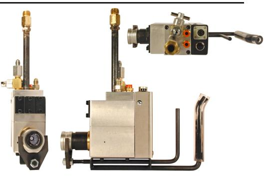
The PCU Series 300 A/C Charging Tool is part of an automated charging system designed to process the A/C system on appliances and vehicles. The system normally consists of a charger which provides a fast precise method of dispensing refrigerant, along with product vacuum checking prior to charging. A line accumulator and/or booster pump which maintain a consistent refrigerant supply.
