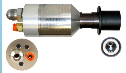
The series 10 coupler is the interface adapter for pressure bleed recovery. When a system is under pressure with helium or another gas, manually clamp the series 10 coupler onto the fitting, and start cycle. System controls will automatically apply air pressure to discharge system. When cycle is complete, the operator will remove BalLoc coupler by pulling on sleeve to release BalLoc Clamping.
