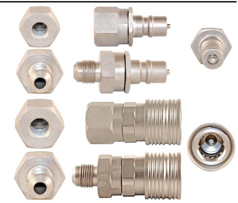
Models 64 and 65 Series 250 is the same flow and internal components as Models 61 and 62 however it is NOT interchangeable. Use these models when there are two fluids or more which should not be mixed. Models 64 and 65 are nickel plated for color difference from Models 61 and 62 which are black in color.
