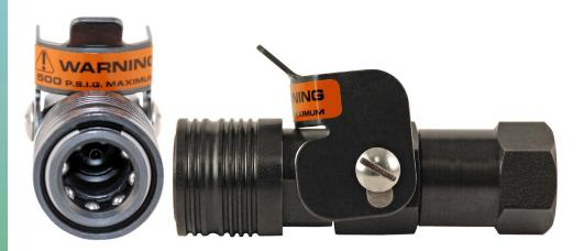
After connecting to the nipple, the operator opens the flow passage and shutoff valve by opening the lever and rotating it in the "up" position. This action locks the tool onto the process nipple preventing release of the tool during processing. When processing is complete, the operator closes the flow passage and shutoff valve by rotating the lever into the "down" position. The tool may then be removed from the process nipple.
