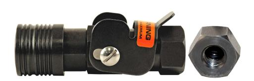
With the operating lever in the closed (down) position, the operator can connect the tool to the process nipple by pulling back on the tool sleeve and engaging the nipple.
