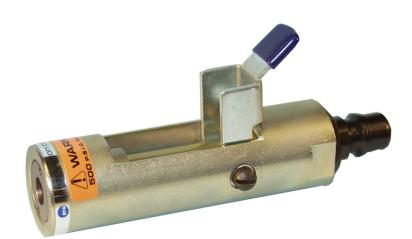
The Production Control Units Series 93 T.Q.C. is designed for easy installation onto the end of either straight or belled type tubing. With an engagement length of one (1"), the actual gripping to sealing length is three fourths (3/4") of an inch. Slide the coupler onto the tubing until seated and then push down the camming lever allowing the shuttle to drive forward causing the collet to grip and tubular seal to seal the process tube for the evacuation, charging or pressure testing.
