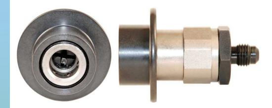
The Production Control Units Series HFC 134a BalLoc Coupler, Model 86, is designed for easy installation onto the SAE J639 low side process fitting. Use the Model 86 Coupler for evacuation or refrigerant charging with de minimus refrigerant loss to atmosphere from the Coupler.
