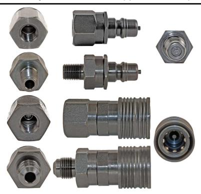
The Models 71 and 72 Nipple and Coupler assemblies have an improved seal design. Field testing has shown that this design will offer longer life and better compatibility characteristics with blended refrigerants and ester oils. They will provide positive leak-tight shutoff and will hold pressure from vacuum to 1000 psig.
